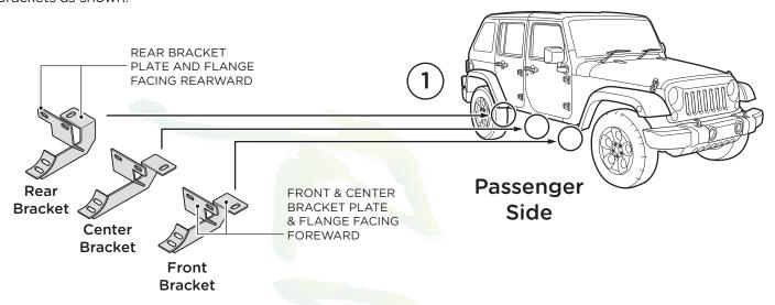
**2.** Starting on the passenger side front, locate the bracket mounting location on the underside of the Jeep body.
