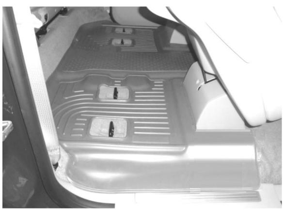
NOTE SEAT ATTACHES TO FLOOR THROUGH LINER
