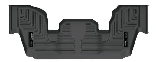
TO EASE INSTALLATION OF YOUR NEW LINER, MOVE BOTH SECOND ROW SEATS TO THEIR MOST FORWARD POSITION. WITH THIS DONE, INSTALL THE LINER AS SHOWN ABOVE. ONCE YOU HAVE INSTALLED YOUR LINER, REPOSITION THE SEATS AS DESIRED.
