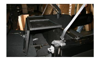
**STEP 5:** ONCE STABLE, MOUNT THE CARGO CENTER PLATE TO THE BACK SEAT PLATE USING (10) 8MM X 35MM BOLTS WITH 8MM LOCK AND FLAT WASHERS. LEAVE SEMI LOOSE FOR ADJUSTMENT.
