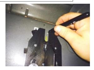
**Step 7:** Remove Nerf Step and set aside. Next, slide the additional 3/8 threaded clip from the upper rectangle hole and align with the "U" shaped mark from step 5. Make a mark through the threaded part of the clip.
