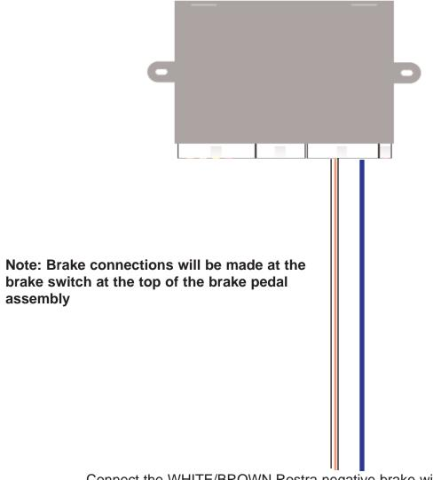
Connect the WHITE/BROWN Rostra negative brake wire to the VIOLET/WHITE at the brake switch of vehicle.
