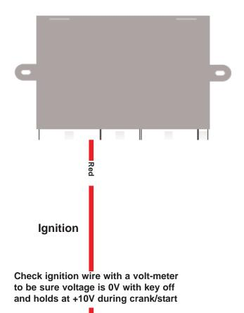
Connect  $\underline{RED}$  wire from cruise harness to  $\underline{BROWN/YELLOW}$  at IGNITION SWITCH 7 PIN CONN, PIN 1
