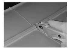
Where applicable, feed the strap through the liner that used to lower your third row seats. Vehicles with power folding rear seats will not have the straps.
