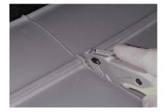
3. To access the LATCH attachment points on the back of the larger 3<sup>rd</sup> row seat back, you will need to trim your liner. Use he recessed trough around the inside bottom of the opening. A utility knife works well for trimming.
