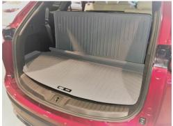
6. The liner at this point is fully installed and is ready to use. If the liner needs to be removed, grab the rectangular Velcro patches and hold them firmly in place as you pull the liner from the seat. This Velcro piece is intended to stay attached to the seat back and cargo floor to reduce wear from the liner being installed and reinstalled for cleaning. Note that the liner includes slots that the seat pull handle will pass through.
