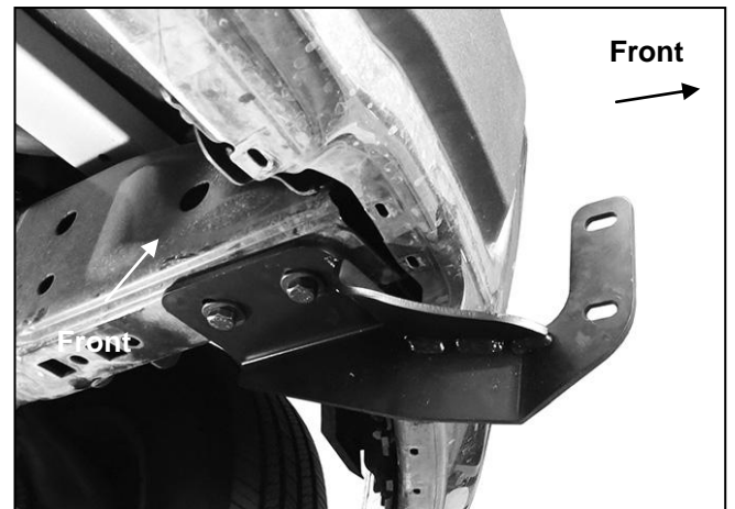
(Fig 16) Attach Frame Bracket to Nut Plate.
