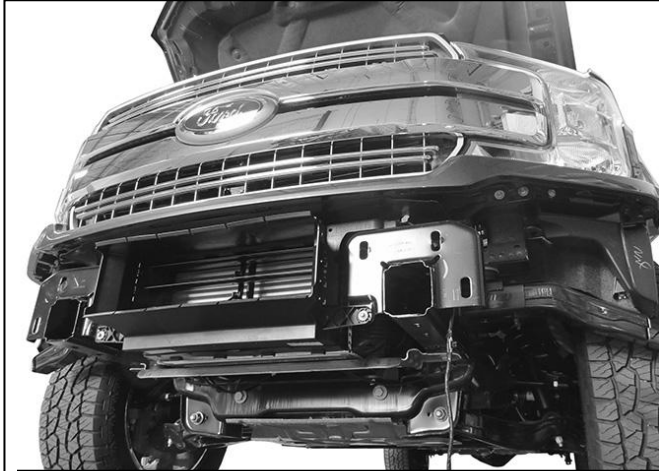
(Fig 18) 2018 models: Remove bumper assembly
