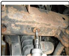
4. If access holes are not present, enlarge the forward most mounting hole on each frame rail so that 1/2" hardware will pass through.
