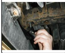
5. Fishwire hardware into position through access holes or holes enlarged in step 4. See FISHWIRE TECHNIQUE on page 2.
