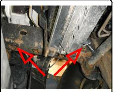
Raise hitch into position and secure to vehicle with 1/2" flange nuts. Torque all 1/2" hardware to 110 ft-lbs.
