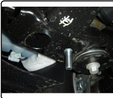
7. Raise hitch into position and secure to vehicle with (5) 1/2" flange nuts.
