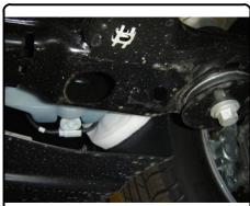
6. Fishwire 1/2" carriage bolts and CM-SP6 spacers into position though access holes into drilled holes. See FISHWIRE DIAGRAM on page 2.
