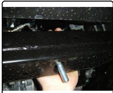
4. Raise hitch into position and mark drill hole locations.
