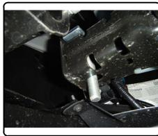
3. Insert 4" hex bolt with 1/2" washer through the top of vehicle cross member. (**Note:** Hoses above the cross member and the strap which holds the hoses may need to be moved slightly to get the hardware into position.
