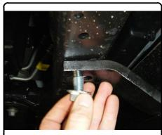
Torque all 1/2" hardware to 110 ft-lbs.Install is complete.
