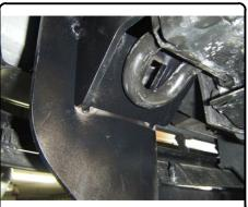
4. Loosely insert the included M10 hex bolts with 3/8" conical tooth washers into weldnuts which bolts were removed from in STEP 2.
