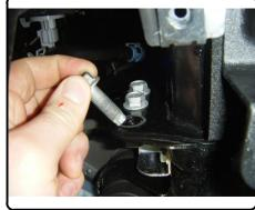
3. Lift hitch into position, locating the vehicle tow loops under the hitch mounting plates.
