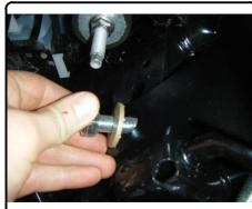
6. Insert 5/8" carriage bolts through the hitch mounting plates and tow loops. Secure hitch to tow loops by attaching supplied spacers and 5/8" flange nuts to carriage bolts.
