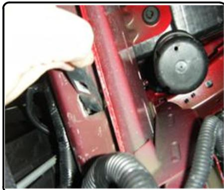
10. Install driver side and passenger side plates and secure with 1/2" hex flange nuts. Using the hitch side plates as a template, drill front holes.
