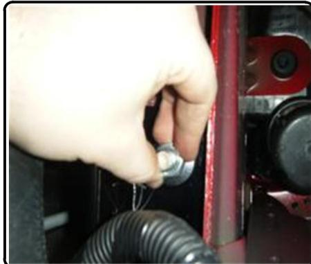
13. Install hitch center section and secure with 7/16" carriage bolts and 7/16" hex flange nuts.
