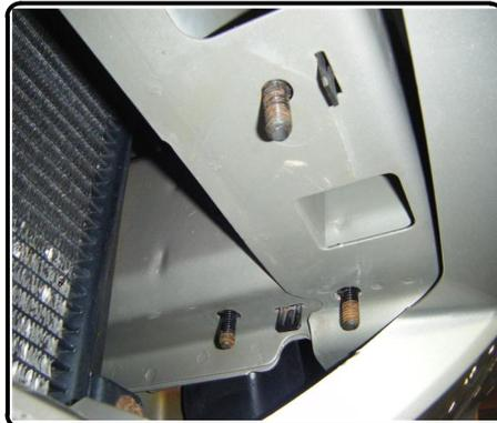
5. Remove the front frame end caps to allow removal of factory installed tow hook hardware.
