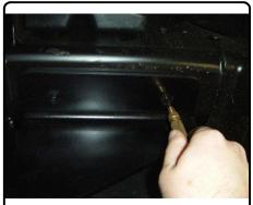
4. Lower hitch and drill (4) 17/32" holes marked in Step (3).
