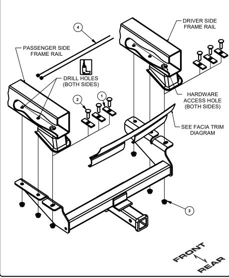
1. Determine if trimming is required on model by raising hitch into position. If needed, mark and trim lower fascia, as shown below, or remove lower fascia and return to owner.
