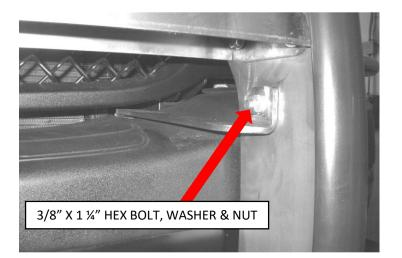
**STEP-8** ATTACH THE GRILLE GUARD ASSEMBLY TO THE UPPER BRACKETS USING THE 3/8 X 1" HEX BOLTS, LOCK WASHERS, FLAT WASHERS AND HEX NUTS.
