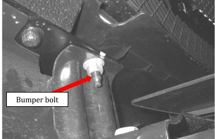
**STEP-2** BEGINNING WITH THE DRIVER SIDE, REMOVE THE NUT AND UPPER BUMPER BOLT. THE BOLT IS LOCATED ON THE BACK EDGE AT THE TOP OF THE BUMPER. THIS LOCATION WILL SERVE AS THE UPPER BRACKET MOUNTING POINT.
