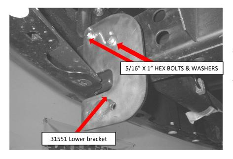
**STEP-7** LOOSELY ATTACH ONE OF THE 31551 LOWER BRACKETS TO THE BUMPER BRACKET USING 5/16" X 1" HEX BOLTS, FLAT WASHERS AND LOCK WASHERS. REPEAT STEPS 5, 6, AND 7 TO INSTALL THE PASSENGER SIDE.
