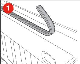
Install the bulkhead seal to the top of the bulkhead at the edge of the bed opening. If the truck does NOT have a drop in bedliner, use 3/4" seal. If the truck does have a drop in bedliner, use 1/4" seal.
