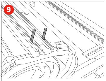
At the front cab, fold the cover back and insert 2 mounting bolts through the keyed slots. Repeat on opposite side.
