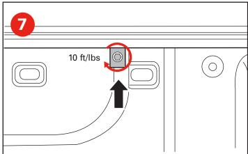
Place the rear clamp as close to the tailgate as possible, should be less than 12". Check all clamps are square and tight with approx 10 ft/lbs of torque. Caution: over tightening the clamp may warp the bed cap.
