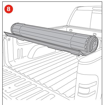
With both rails clamped in place, rest the roll top on the rails at the tailgate, roll forward into the opening and remove and discard all packaging materials.
