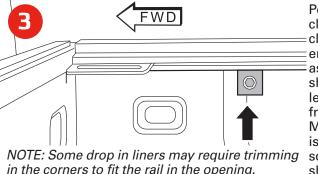
Position clamp as close to the end of rail as possible, should be less than 12" from the end. Make sure rail is clamped square as shown.
