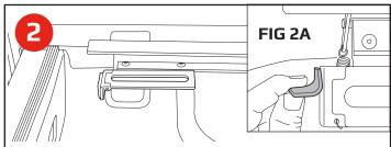
Position Revolver rail with the silver slotted bracket all the way forward towards the cab of the vehicle. If the truck is equipped with a drop in bedliner remove the foam pad located on the slotted bracket as shown in Fig. 2a.
