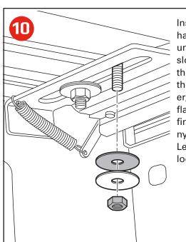
Install mounting hardware loosely underneath the slotted bracket on the rail. Start with the rubber washer, then the large flat washer, then finally add the nylon lock nuts. Leave the nuts loose for now.
