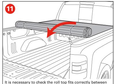
It is necessary to check the roll top fits correctly between the rails. Roll the cover from front to back and back to front to verify it rolls freely on the rails.
