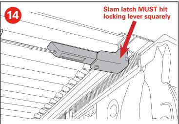
When correctly installed, the vinyl edges of roll top align squarely with the rails in the 4 corners. The latch assembly will align with the silver locking levers at the tailgate on each side.
