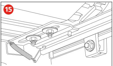
Once properly aligned, roll the cover open ensuring you DO NOT misalign the roll top. Tighten the nylon lock nuts at the front. Recheck the roll top operates correctly. When latched, check the locking rails prevent the cover from lifting on both sides.
