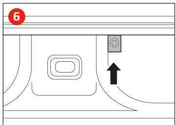
Place the 2nd clamp near the center of the rail. See steps 4 and 5 to ensure the clamp goes on correctly. (8' beds-evenly space 2 clamps between ends).
