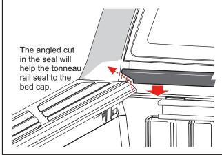
As you adhere the bulkhead seal, match the other end to the bed cap and trim it also to fit the cap's edge.
