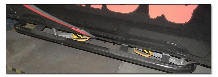
**Step-6** Repeat the installation steps to install the mounting brackets and step on the driver side.
