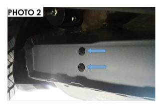
5. Attach the front bracket on the threaded hole and secure with (2) M8 x 30mm. Hex head bolt (2) M8 flat washer and (2) M8. Lock washer, Photo 3. Attach the central bracket on the threaded holes and secure with (2) M8 x 30mm. Hex head bolt, (2) M8 flat washer and (2) M8. Lock washer. Photo 4. Attach the rear bracket on the threaded holes and secure with (2) M8 x 30mm. Hex head bolt (2) M8 flat washer and (2) M8. Lock washer. Photo 4.
