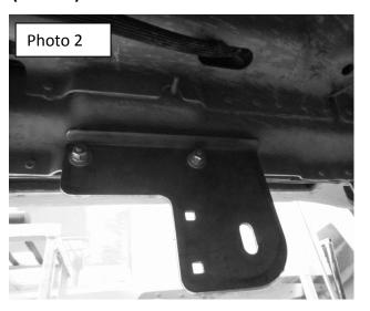
2. Install the auxiliary bracket using (1) b M8 hex nut Gray P., (1) 5/16" flat washer Gray P. and (1) 5/16" spring lock washer Gray P. Then attach the auxiliary bracket to the front bracket using (2) 5/16" carriage head bolt Black P., (2) 5/16" flat washers Black P., (2) 5/16" spring lock washers Black P. and (2) 5/16" hex nuts Black P. Leave loose for final adjustment. (Photo 3)
