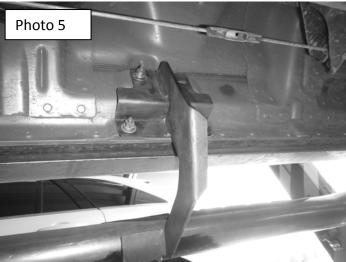
4. Locate the three M8 welded bolts in the rocker panel near the end of the cab. Install the rear bracket using (3) 5/16" flat washers Gray P., (3) 5/16" spring lock washers Gray P. and (3) M8 hex nut Gray P. Leave the nuts loose for final adjustment. (Photo 6 & 7)
