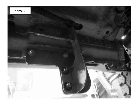
3. Locate the three M8 welded bolts in the rocker panel at the middle of the cab. Install the center bracket using (3) 5/16" flat washers Gray P., (3) 5/16" spring lock washers Gray P. and (3) M8 hex nut Gray P. Leave the nuts loose for final adjustment. (Photo 4 & 5)
