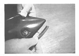
STEP 2: Attach the included rubber seal to the Fender Flares, Peel back 2" of the adhesive backing and position on the Fender Flare. Attach the seal to the Fender Flare, peeling back a few inches at a time. Ensure pressure is used to secure rubber seal to Fender Flare edge, Attach rubber seal along the top leading edge of the Fender Flare where it will make contact with the vehicle body.
