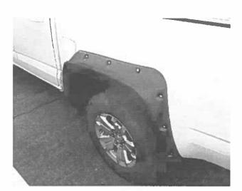
**STEP 9:** Repeat installation method for other side. Double check the front Fender Flares to make sure all bolts are tight and clips are securely fastened. Your installation is now complete. Do not use abrasive cleaners.
