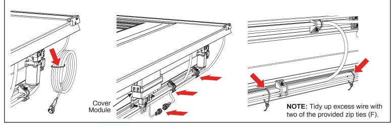
Before routing the main wiring harness (E) from the bed to the battery, first locate your battery in the engine compartment. Determine which side of the vehicle the battery is on - passenger or driver side - and then route the main wiring harness on the same side as your battery. Feed the battery terminal connection end of the main wiring harness (E) into the available pickup bed hole. Bring the wire down between the bed and the cab.
