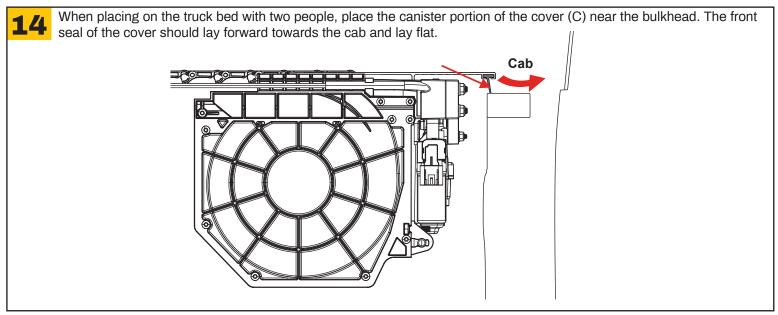
With the cover (C) in place, the front seal lays flat on the bulkhead, but must not extend past the bed rail cap. Trim the seal as needed to ensure that it lays flat.
