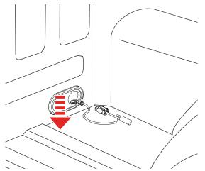
**NOTE:** Make sure to leave enough wire harness in the bed to attach to the cover module later
