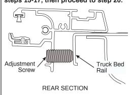
If the rails measure to be too close together, turn the screws counter clockwise.
