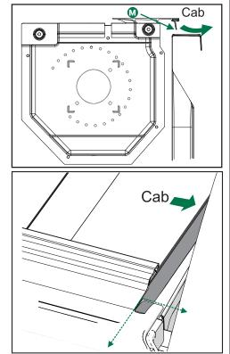
**Position the rails:** Move the cover back toward the tailgate and use the shipping bracket as a spacer to position both rails to be 1/8" from the tailgate.
