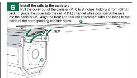
Fasten the rails to the canister:
