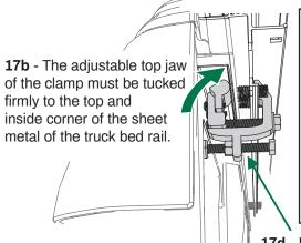
17c - If the jaw does not contact firmly into the corner of the bed flange, remove the clamp and loosen the screws to adjust the jaw.
