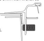
If the rails measured too close together, turn the screws counter clockwise.
