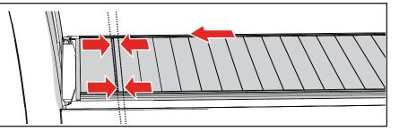
Remove the protective film and install the drain tubes:
