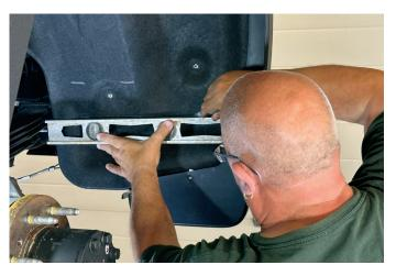
16. Cut the liner along the horizontal line made.
