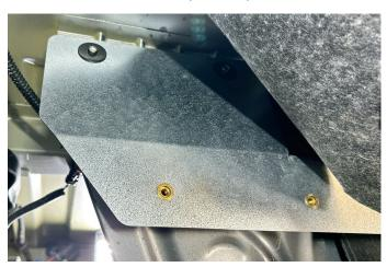
25. The bracket should now be installed & look like this. Ensure outer part of bracket is installed behing the wheel lip.
