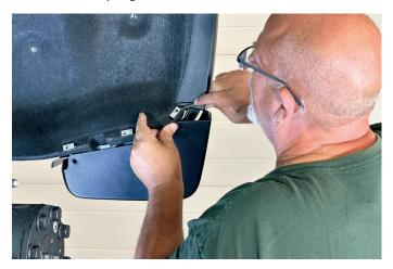
5. Reinstall spring nuts on the sheet metal as shown.
