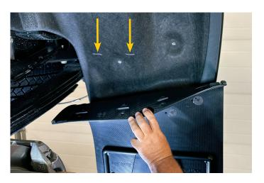
12. Roughly line up to 2 left lower holes of the bracket with the marks made & mark below the bracket with a marker.
