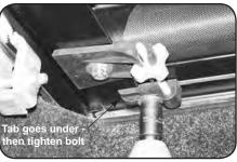
E. Then tighten bolt (left loose earlier) under front bar on each tension adjuster.
