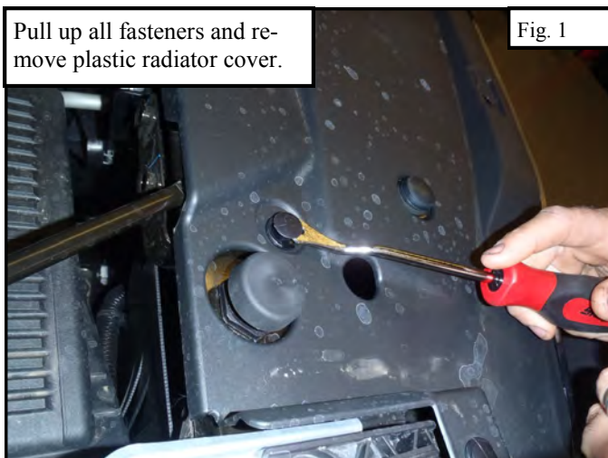
Remove the two fasteners on each side attaching the filler panel to the body.
