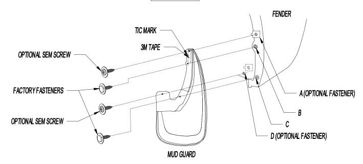
NOTE: Turn wheels all the way left or right for easier installation. It may be necessary to remove the wheels before mud guard installation.
