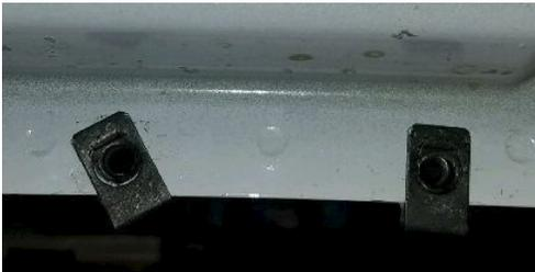
Slide 2 clip nuts on the pinch weld for lower holes. Attach the AC bracket using (2) 8MM Bolts and (2) 5/16 Lock Washers on the bottom Clip Nuts and (2) 5/16 Thread Cutting Bolt and (2) 5/16 lock washers on the upper holes
