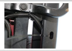
Cut the cable ties on the 4-flat portion of harness and route it down through the opening behind the taillight.
