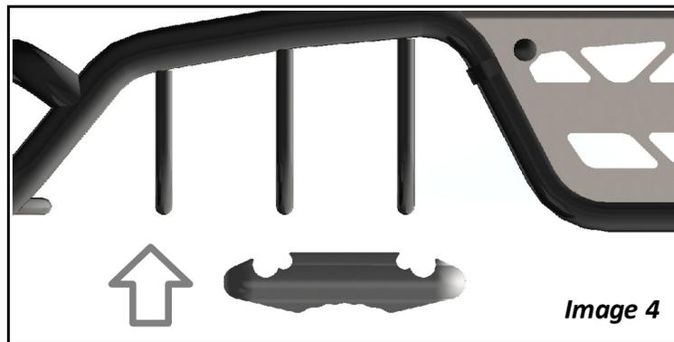
**4.** Place the Safari Rack with the plastic holders above the roof bars of your vehicle\*. **Note 1:** It may be necessary to slide and relocate the roof bars to allow the installation.
