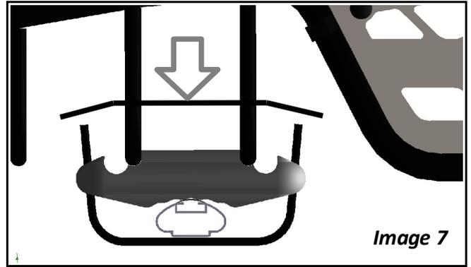
6. Secure each thread of the “U”-bolt with a Knob nut.
