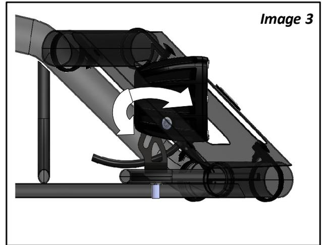
**3. Install safari rack.** Place the (x4) plastic holders below the safari rack and close to the edges. Distribute them at the same distance from center then snap them between the cross tubes.
