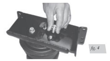
5. Attach the lower bracket (C) to the air spring (A) with flat washers (M), lock washers (N), and 3/8" X 7/8" hex head bolts (L). Refer to Figure 5. Tighten to 20 lb.-ft.
