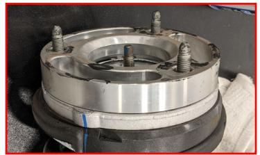
Re-install the shock to lower control arm bolts. Do not tighten. Using the jack under the lower control arm, raise the arm up until the shock studs are protruding through the frame holes in the shock tower.
