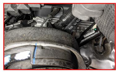
Remove shock to lower control arm bolts. Retain factory hardware.
