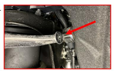
Install the ride control relocation bracket on the upper control arm using the supplied M6 button head allen bolt.
