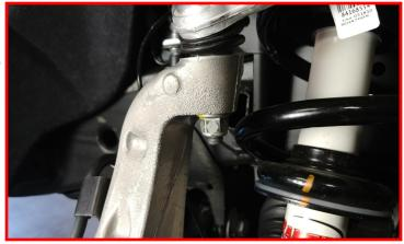
Install the brake line bracket from the upper control arm using the factory hardware. Torque to 5 ft-lbs.
