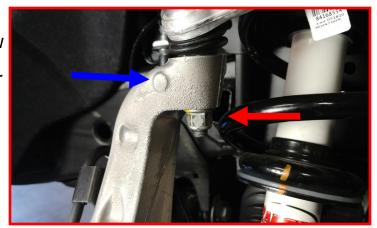
Loosen but do not remove the lower control arm mounting hardware. Locate the lower shock bolts and remove. The shock may "pop" outboard when removed due to the angle of the control arms.
