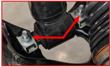
Install the provided M10x1.5 short nuts to the shock studs. Torque nuts to 35 ft-lbs.
