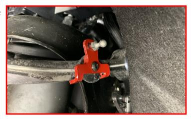
Install the ride control linkage on the ball stud by pushing the linkage back onto the ball stud.
