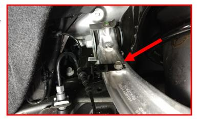
Loosen the upper control arm to knuckle nut but do not remove. Using a dead-blow sledgehammer, strike the upper ball joint boss to loosen the taper joint. When taper joint is loosened, remove nut and let knuckle hang. Retain factory hardware.
