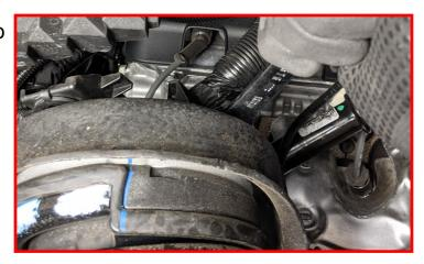
Torque shock to lower control arm bolts to 45 ft-lbs.
