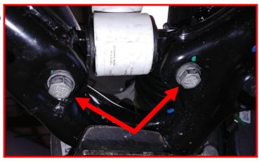
Install the factory nut on the sway bar end link. Torque sway bar end link lower nut to 45 ft-lbs.
