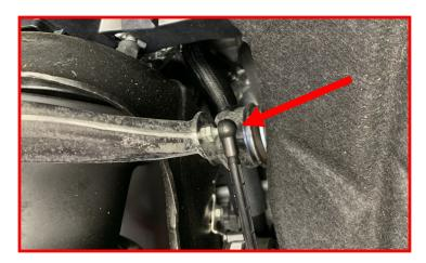
Remove the ride control linkage from the ball stud on the control arm.
