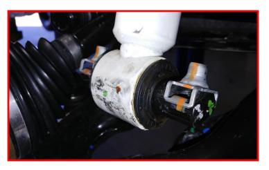
Remove shock assembly from vehicle and install ReadyLIFT spacer to the shock top mount.
