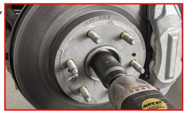
Using a dead blow sledgehammer, strike the end of the axle until it moves back and forth freely. Remove axle nut at this time, be sure to retain the axle nut for later installation.
