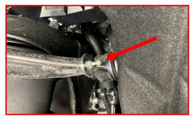
Remove the ball stud from the upper control arm. Retain the ball stud.
