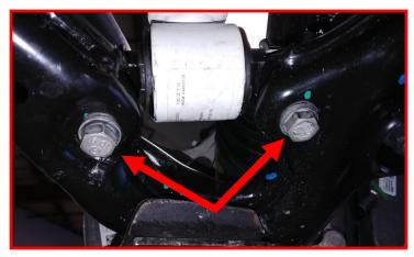
Remove lower sway bar end link nut. Retain factory hardware.
