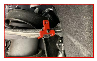
Install the ball stud in the rear hole of the ride control relocation bracket using the supplied 6MM lock nut.
