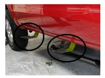
**Step-3** Attach the front bracket to the rocker panel using the install (2) M10 Hex nut (2) flat washer and (2) lock washer. (Photo 3).
