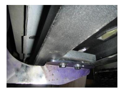
**Step-5** Align the running board with the vehicle and tighten all brackets and side steps nuts and bolts. Repeat the above steps to install the passenger side brackets and running board. Remember to check and retighten the nuts and bolts every six months.
