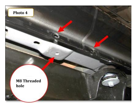
**Step-4** Attach one of the driver side Front/Center brackets to the pinch mold using (2)  $\frac{1}{4} \times 1^{n}$  hex. Head bolt, (4) 1/4" Flat washer, (2) 1/4" Lock washer and (2)  $\frac{1}{4}$ " hex nut, and to the underside of the body using (1)M8 SEMS bolt. **Photo 5 & 6.** Leave the nuts and bolts loose for final adjustment.
