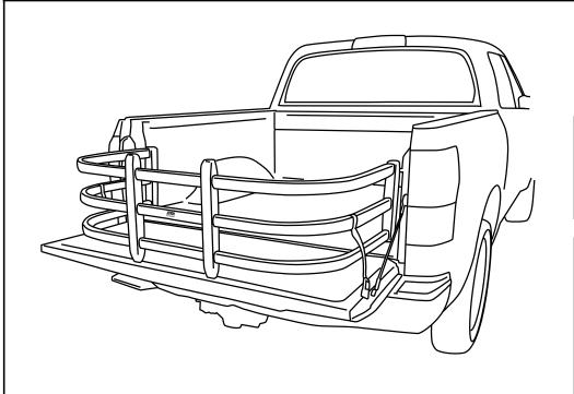
BEDXTENDER HD<sup>™</sup> shown assembled and installed on truck.
