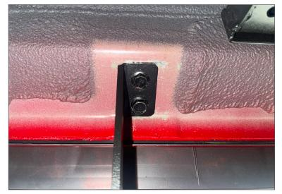
Step 5. Next, tighten the three lower bolts first following with the three upper bolts (15-20 ft./lbs. torque).
