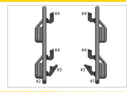
Step 2. Remove OE boards if equipped and discard. Clean any dirt or debris from mounting holes and surface. Step 3. Beginning with the (#1)driver side, carefully raise step rail into place and match the brackets with the factory mounting locations. Next, starting with the center bracket and using the supplied (#5) M8X30mm Hex cap with washer, start and leave loose.
