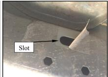
2. Place Stud/nut plate onto the slotted hole (Item 7) as well as the hex riv-cert (Item 8) onto the hexagon hole. (Before inserting stud/nut plate onto the slot place a square plastic retainer (Item 23) on the stud portion of the plate to prevent the plate from falling in the slot, as shown in picture below).
