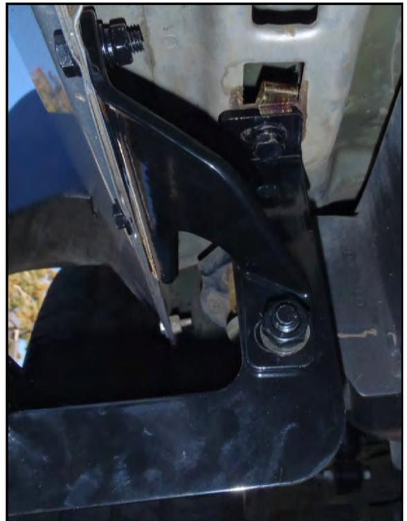
3. Attach the driver front mounting bracket to the vehicle underbody using (x1) M8 hex cap screw, (x1) M8 split lock washer, and (x1) M8 flat washer.
