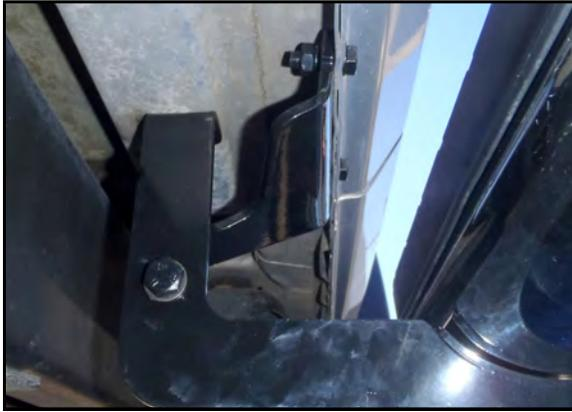
6. Repeat steps 3-5 for the driver center and rear mounting bracket and support bracket. Do not fully tighten at this time.
