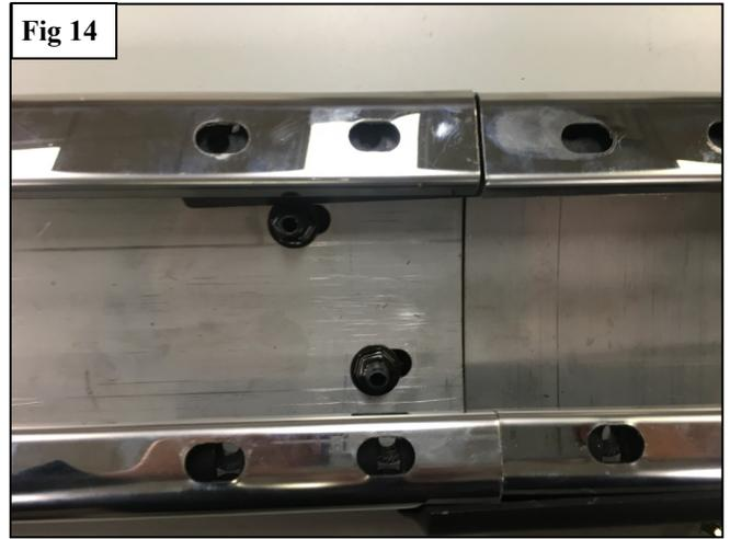
14. Obtain the Link Plate (6) and secure it to the Step Bar Assembly (1 & 2) using the supplied black M6 Hardware. **See Figure 15.**
