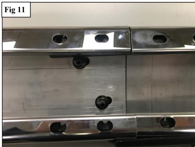
10. Obtain both sections of the Step Bar Assembly (1 & 2). Slide the Reinforcement Links (6 & 7) into both sides of the step bar sections. See Figure 12.
