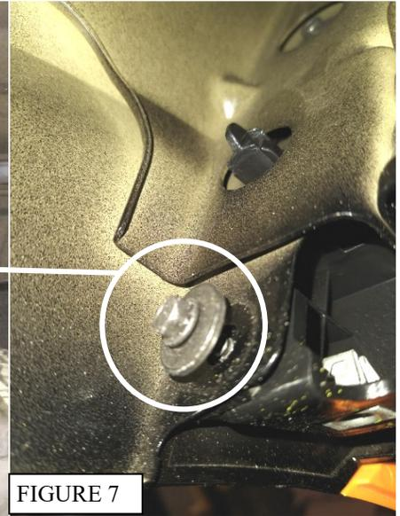
7. With help disconnect any connection from the fascia to the vehicle and carefully disengage the whole front fascia.
