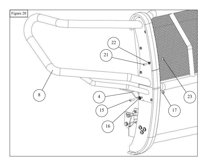
20. Align and adjust the Grille Guard Base, HDX Wings, and mounting brackets as necessary. Tighten and then torque all hardware as specified: M8 to 15-18 ft. lbs., M10 to 35-40 ft-lbs., and M12 to 55-60 ft-lbs.
