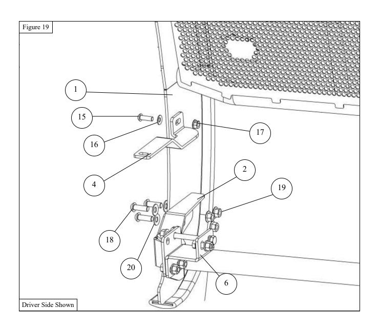
19. Using supplied M8 hardware and the M10 hardware used to mount the upper support strap, loosely assemble the HDX Driver and Passenger Wings to the Grille Guard Base. See **Figure 20** for reference.
