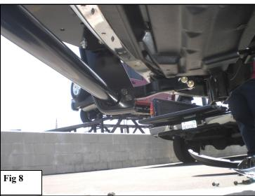
12. Align and adjust the grille guard as needed. Fully tighten all hardware at this time. Torque all M12 hardware to 50-55 ft lbs.
