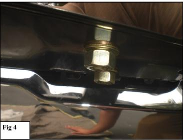
5. Align and adjust the winch tray as needed then fully tighten all hardware at this time. Torque all M12 hardware to 50-55 ft lbs and M10 to 40-45 ft lbs.
