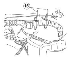
Attach wire harness to the control box. Slide controller through cable ties. Line up cable ties with grooves in controller and tighten. (8)
