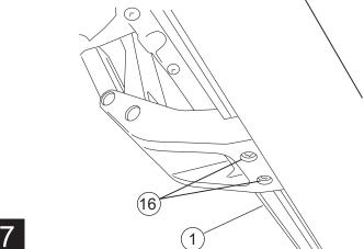
The rearward edge of the board should be about 9.5in from rear mount. Tighten 1/4-20 bolts to 10 ft-lbs.
