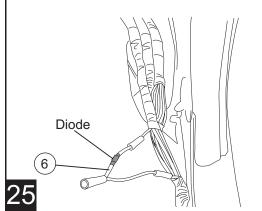
Connect purple trigger wire to Double Diode Harness. Connect one open end of the harness to the red connecting wire from the door and the other end to the blue butt connector of step 25.
