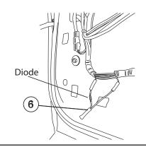
Pass supplied red connecting wire from door to cabin through the door hinge wire accordion. You may want to use the supplied plastic tubing to help pass the wire through.
