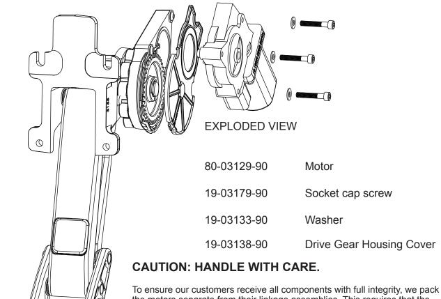
To ensure our customers receive all components with full integrity, we pack the motors separate from their linkage assemblies. This requires that the installer position and fasten the motor before continuing with the install. Please follow the instructions below and handle the assembly carefully.
