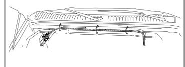
Route harness end with motor connectors down the inner side walls of truck and down along the frame to the motorized linkages. Plug connector into motor.
