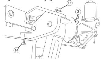
Position idler linkage assembly in forward mounting position and bolt to bracket and drilled mounting holes. Snug all bolts... do not
