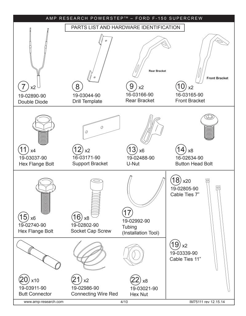
Install U-Nut. Drilling Rear Mounting Holes: Position and clamp drill template as shown, (center on U-Nut) and pilot drill mount holes with 1/8" drill bit. Remove template and drill holes to 21/64".
