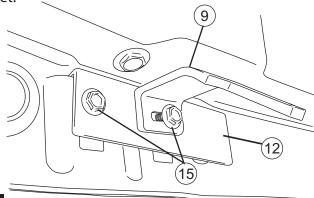
Mount Front Bracket to upper stock mounting hole that the drill template was centered about.
