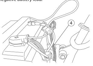
Route the long end of the harness along firewall and secure with tie wraps along the way.
