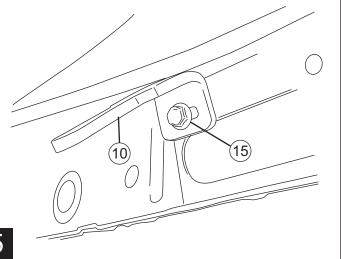
Install U-Nut. Drilling Forward Mounting Holes: Position and clamp drill template as shown, (center on U-Nut) centering the template around stock mounting hole.
