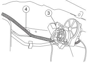
Pierce holes in front floor board grommets to allow access for harness trigger wire into cab of vehicle. Push purple trigger wires through pierced holes.
