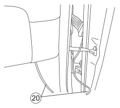
Connect door end of red connecting wire to the blue butt connector of step 22. Secure any loose wires with tie wraps and/or electrical tape.
