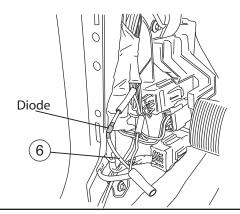
Locate harness bundle under driver sill plate, open bundle and find Black with Light Blue stripe wire. Splice into wire single diode harness with the diode end toward the front of the vehicle.
