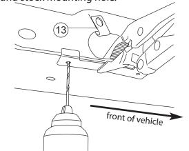
Position Drive Mount at rear mount location and bolt to bracket and drilled mounting holes. Snug all bolts... do not fully tighten.
