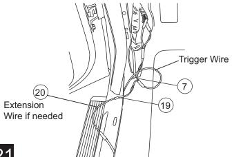
On the Passenger side remove front door paneling and locate wire bundle running out toward the door latch as shown. Connect Single Diode Harness to Black with Pink stripe wire with diode end heading back toward the vehicle cabin.
